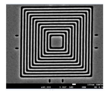
photomicrographs. Please note the contrast depends upon illumination and is not particularly high. For instruments with verniers or electronic calipers distance measurements can be verified using a pitch pattern of appropriate size. The standard is ideal for measuring modulation transfer functions.
