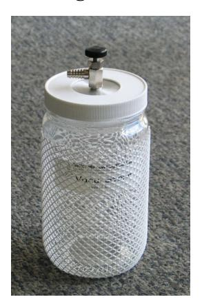
The Vacu-Storr series of glass vacuum containers were developed to store materials which sensitive to moisture, oxygen, and other gases found the environment. It can also be used to protect the environment from the contents. Also available in stainess steel. The Vacu-Storr is capable of nearly reaching the vacuum level of  $10^{-4}$ torr. With higher a conductance valve and capable pump 10<sup>-6</sup> torr is achievable.
